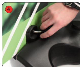
Place the thumbscrew through the graphic holder and tighten until fully secure.
