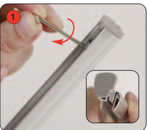
1 Using the Allen key supplied with the user instructions, loosen the top rail screws. Rotate the rail end cap to expose the steel flat bar.
