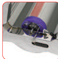
Tensioner built into roller mechsanim
